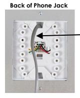
3. Run the phone cable behind the aluminum plate and up through the back of the RJ11 phone jack.
