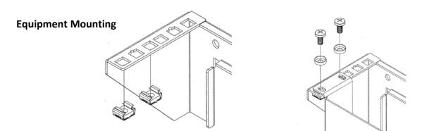
1. Install M6 Cage Nuts into the square openings to provide an attachment point for the M6 Mounting Screws.
