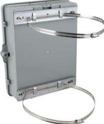
The image shows a silver metal enclosure with two metal brackets attached to its top and bottom edges. Each bracket consists of a flat base with a curved, hook-like top section, designed to wrap around a pole. | The Altelix NMKG-240-08 Pole Mount Kit easily attaches to the enclosure. This pole mount kit allows the enclosures to be mounted to poles up to 7.6 inches in diameter. The mounting brackets are constructed from 0.04" (1mm) thick galvanized steel for all weather applications. |
