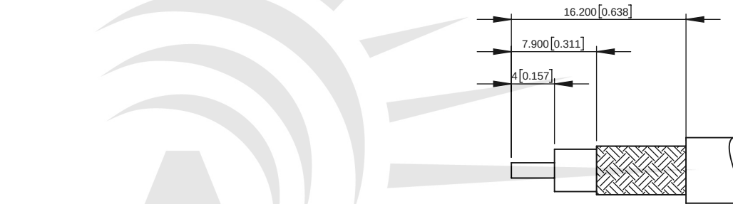
RG-8X RECOMMENDED CABLE STRIPPING DIMENSIONS
