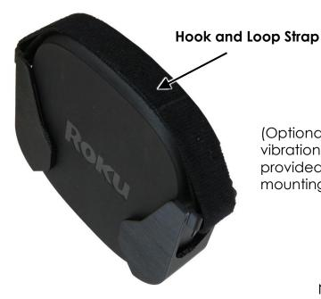
(Optional Step) For installations subject to vibrations, an optional hook and loop strap is provided to secure the Roku Ultra in the mounting cradle.
