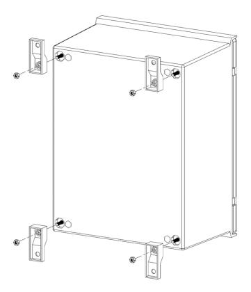
The provided mounting feet can be used to mount the enclosure to most surfaces or you can use the appropriate Altelix pole or wall mount kit sold separately on our website.
