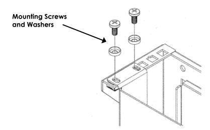
2. After installing the required cage nuts, use the included M6 Mounting Screws and M6 Washers to secure your equipment.
