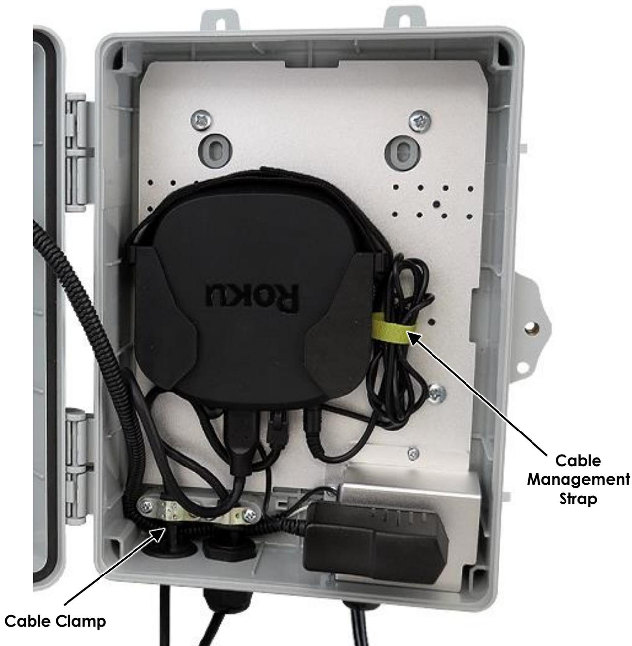
6. Connect the Roku Ultra's power supply to the internal 120VAC power outlet. Secure any loose cables using the cable management straps provided in the accessory kit.
