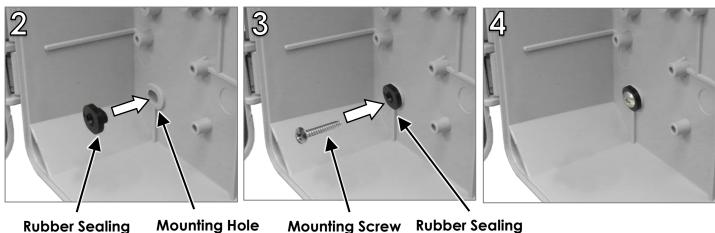
4. When mounting the enclosure, ensure the rubber sealing washers completely cover the enclosure mounting holes to provide a water-tight seal. Silicone sealant can also be added to enhance the seal.
