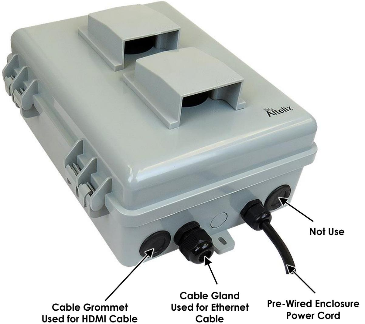
3. Run the HDMI cable into the enclosure through the cable grommet shown. Carefully cut a slit into the grommet and then feed the HDMI cable into the enclosure.
