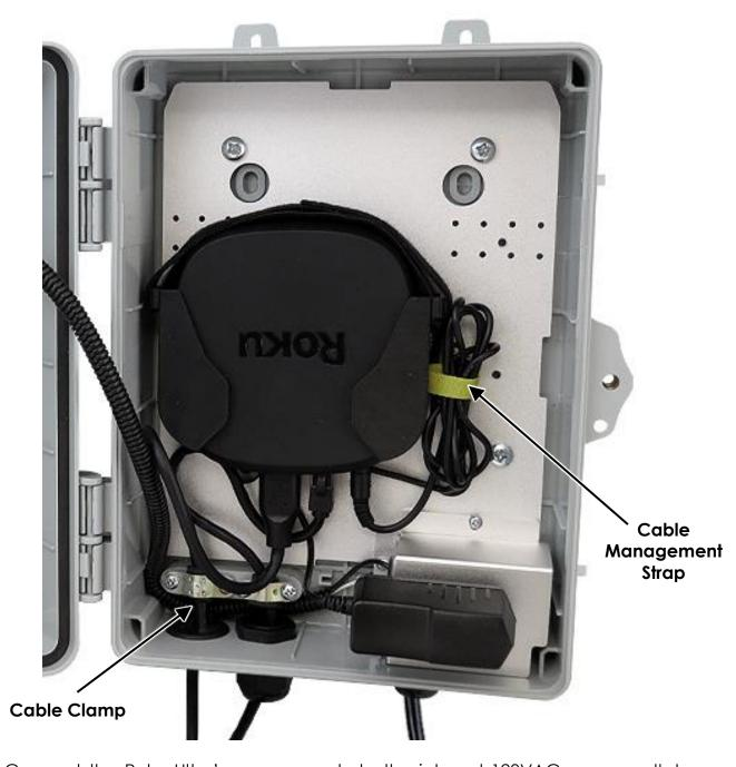
6. Connect the Roku Ultra's power supply to the internal 120VAC power outlet. Secure any loose cables using the cable management straps provided in the accessory kit.
