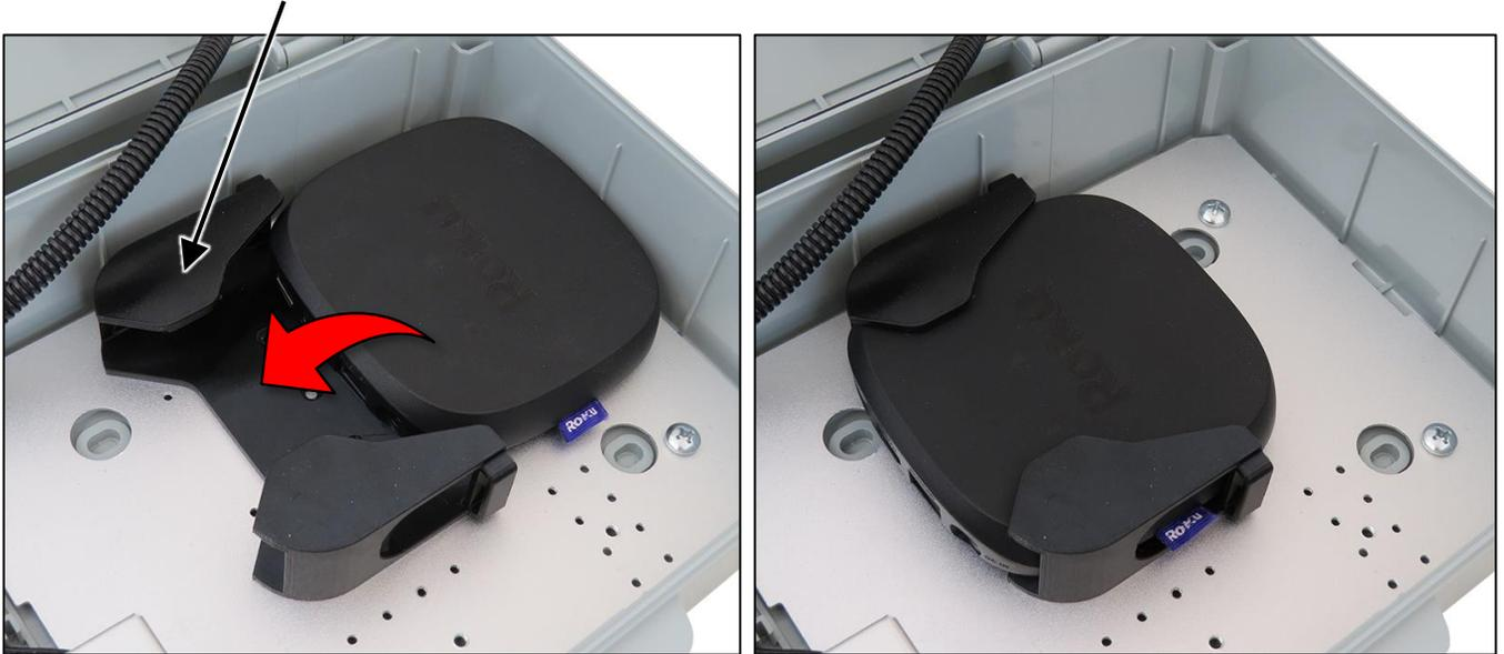
2. (Optional Step) For installations subject to vibrations, an optional hook and loop strap is provided to secure the Roku Ultra in the mounting cradle.
